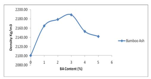
Figure 4: Variation of Density (Kg/m3) with Modifier Content
