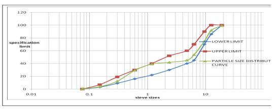
Figure 1: Aggregate Gradation Curve
