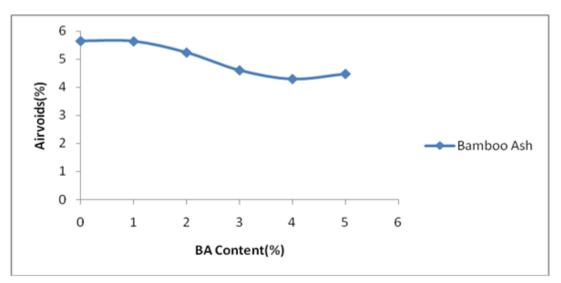
Figure 5: Variation of Air Voids with Modifier Content
